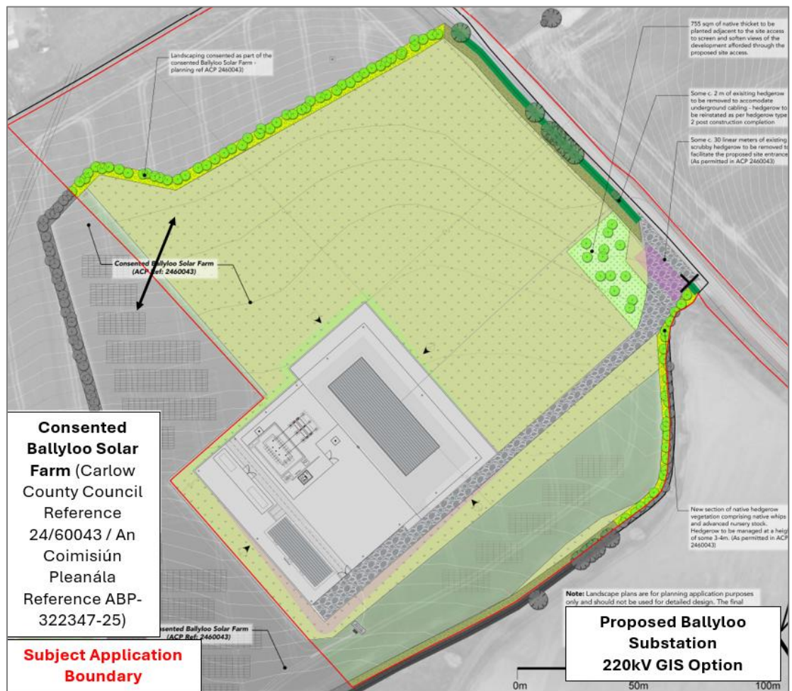
Figure 04: Proposed 220kV GIS Substation Option
